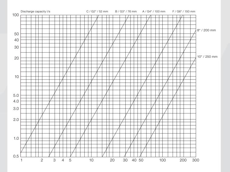
Smooth, internally rubberized hose - Water at 20 °C Pressure loss in m water column per 100 m of hose
