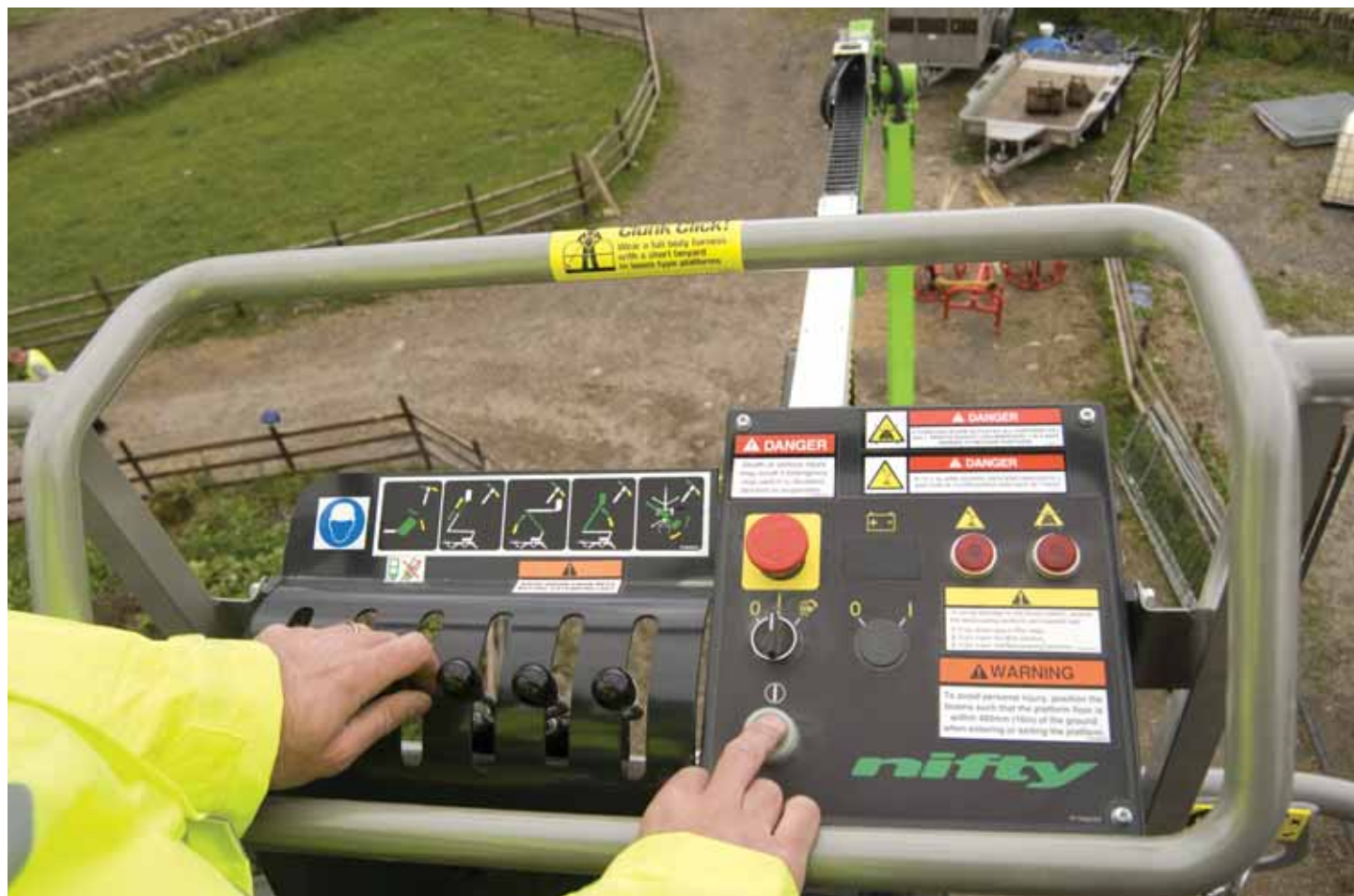
Right and Below: The well-proven Niftylift controls in the basket and on the boom are simple and can be operated with gloves on in the winter.
