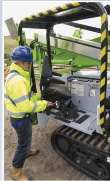
Above: The operator can swing the seat around to face either direction, making it easier to position the prime mover in confined spaces
