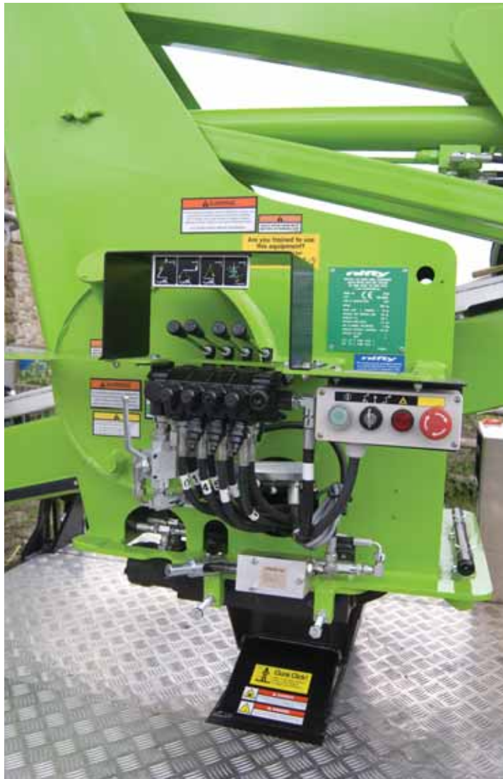
Right and Below: The well-proven Niftylift controls in the basket and on the boom are simple and can be operated with gloves on in the winter.
