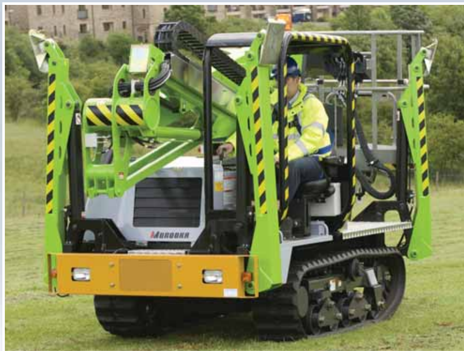
Main Picture and Above: The Morooka can tackle mud and slopes, with a light footprint through rubber tracks that also make it ideal for travelling across higher-value turf.
